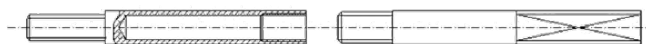
Figure 6 A sketch of the microtorque bar and components. Actually a two parts set, the left hand side one is a thin wall aluminum tube.
